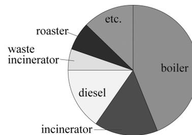
Figure 10. Emission ratio of nitrogen oxides from stationary facilities
