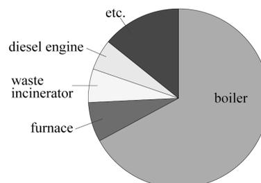
Figure 12. Emission ratio of sulfur oxides from stationary facilities
