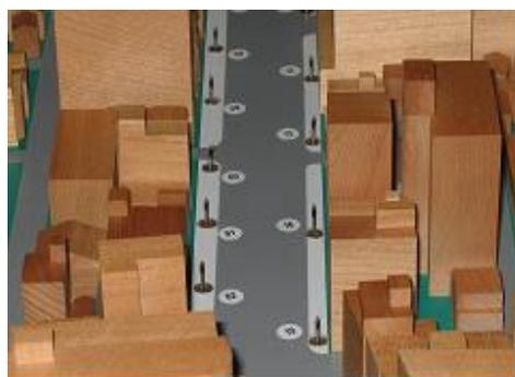
Figure 15. Multi-channel thermister anemometers installed in building models
