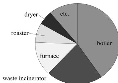
Figure 11. Emission ratio of soot and dust from stationary facilities
