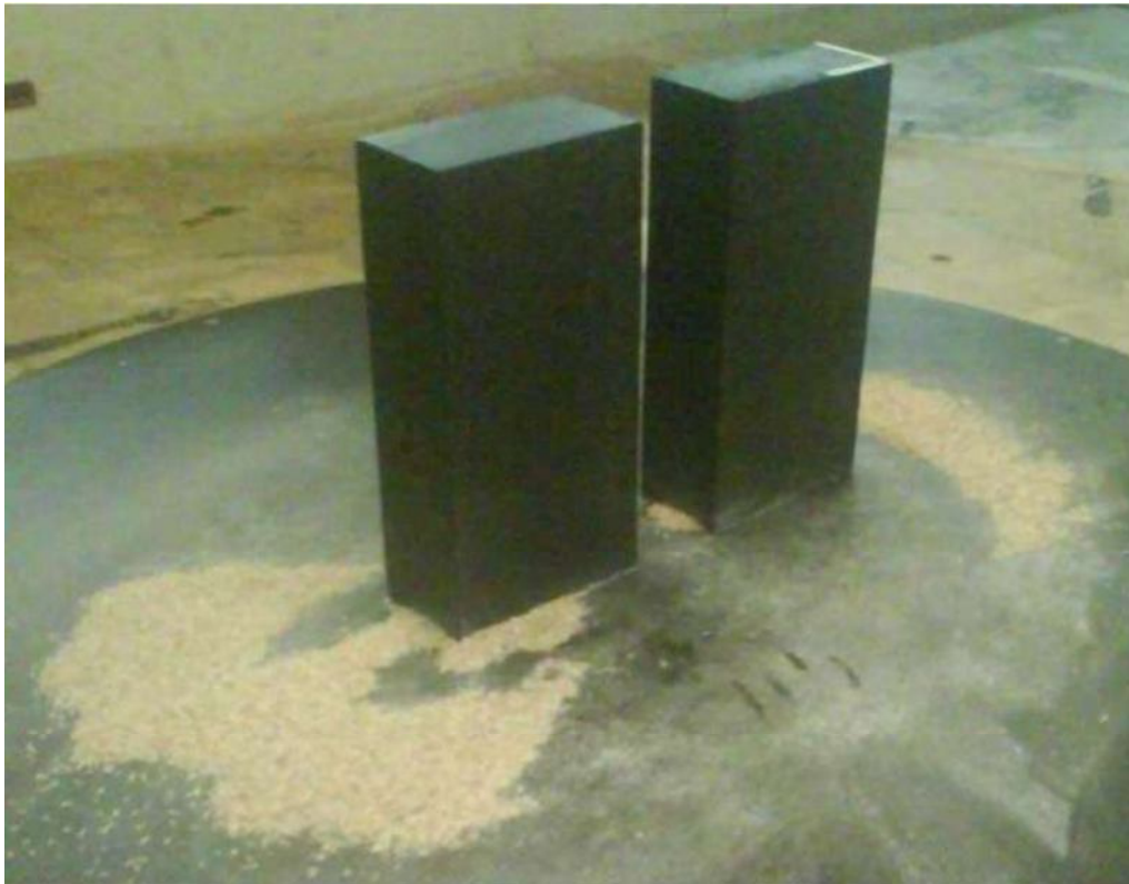
Figure 6 The 1:400 scale models in the wind tunnel during a bran erosion test.
