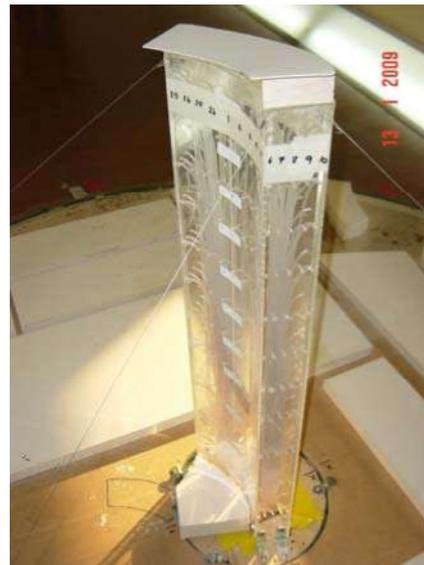
Figure 7. Rigid model of Knightbridge building in Manila
