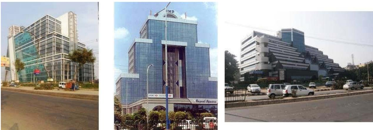
Photo.7 Positive configurations of buildings in Delhi and Gurgaon for reducing the effect of downwash.
