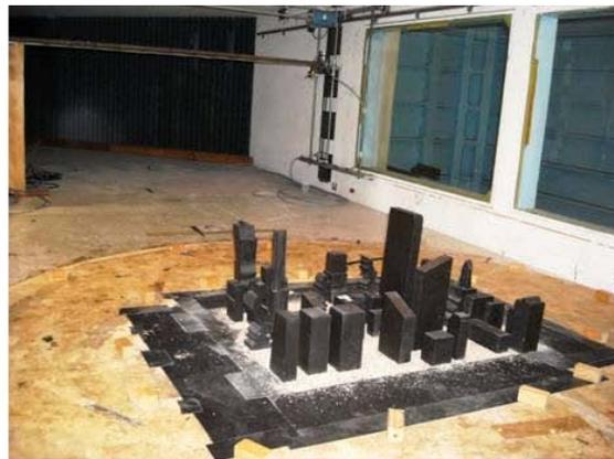
Photo.10 Upstream( left) and downstream( right) views of model in wind tunnel with the addition of bran
