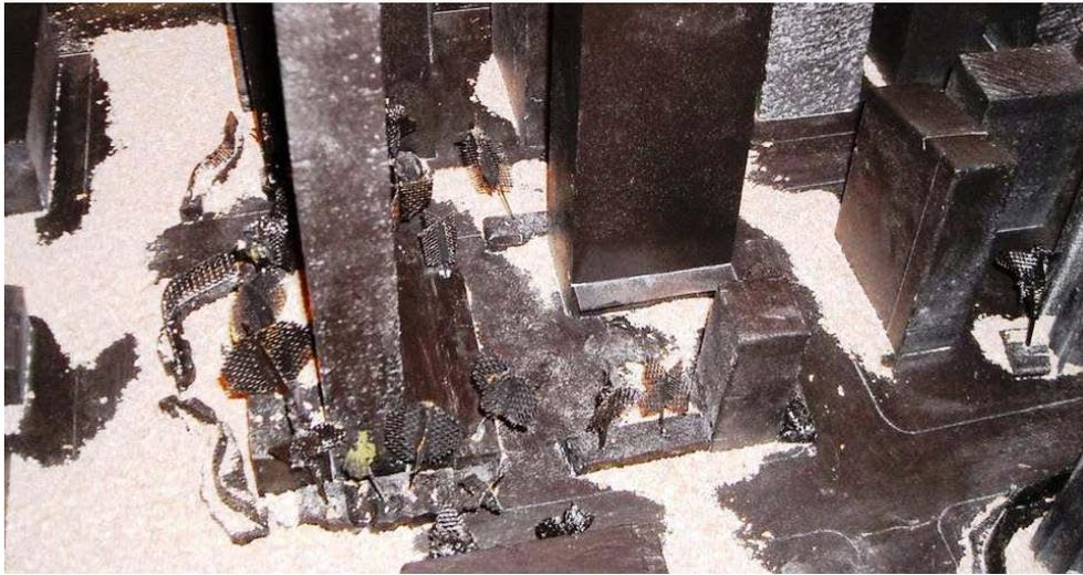
Photo. 13 Erosion patterns after the addition of mitigation features
