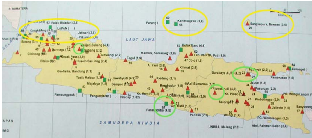
Figure 3. Wind Environment of Jawa Island (courtesy of LAPAN): Yellow < 3.8m/s, Green 3.9m/s -4.9 m/s, Orange 5.0m/s- 5.8 m/s, Red > 5.8m/s.
