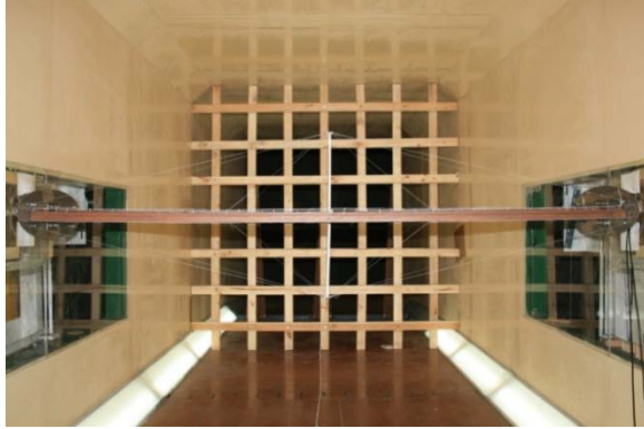
Figure 19 IRR bridge model and grids to generate turbulent flow in wind tunnel
