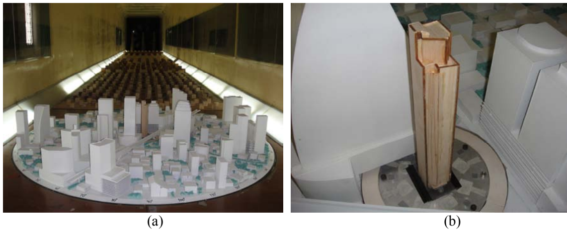
Figure 13. (a) Overall wind load study of Ramada Bangkok Sukhumvit Project by wind tunnel test, and (b) high-frequency force balance model
