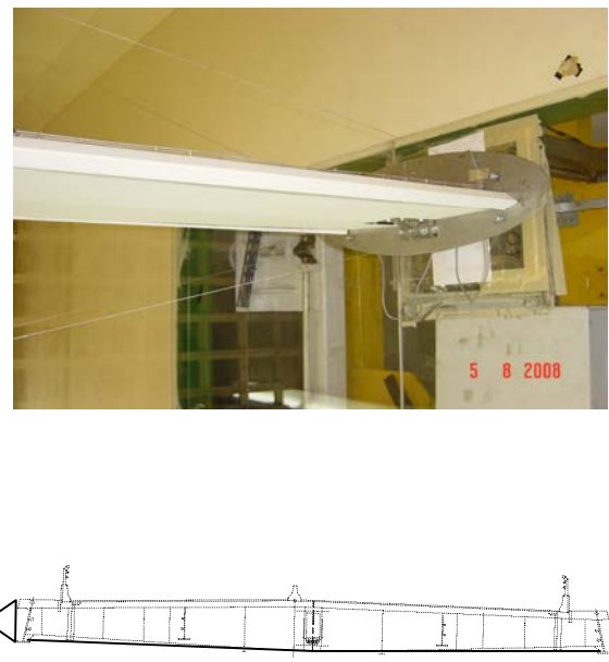
Figure 16. Fairings and soffit plates modified section in wind tunnel
