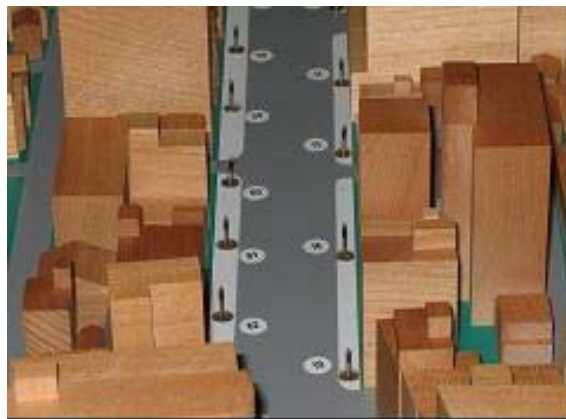
Fig. 1 Multi-channel thermistor anemometers installed in building models.
