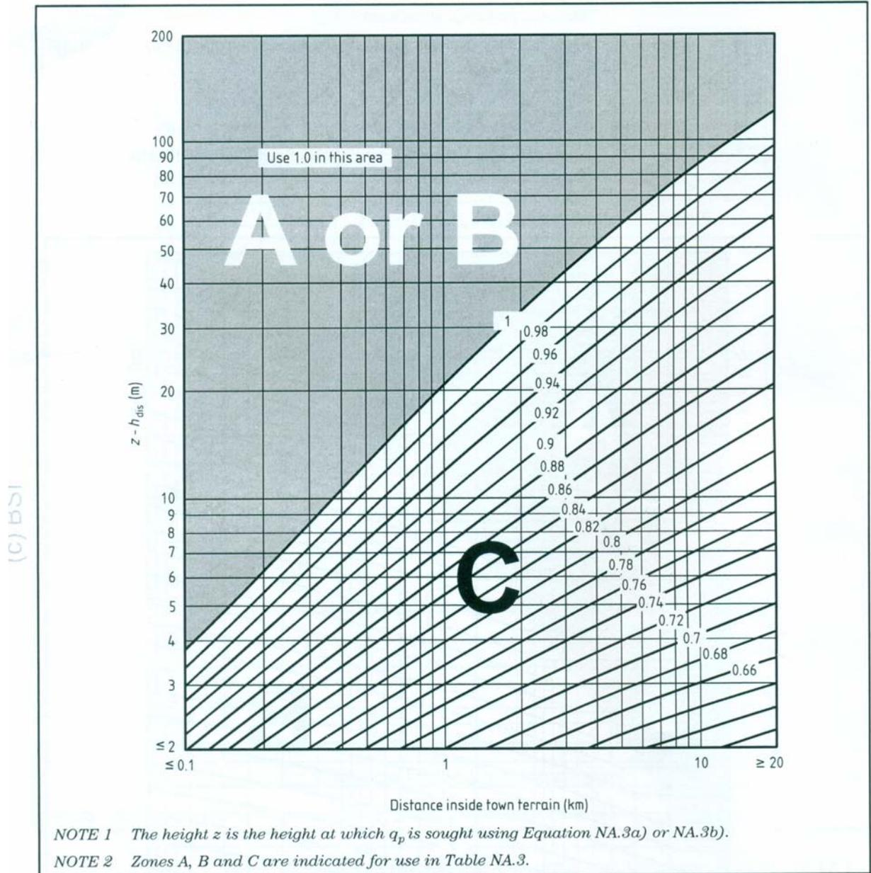
Figure 8: Values of exposure correction factor ( $c_{e,T}$ ) for town terrain (Figure NA.8 of NA to BSEN 1991-1-4:2005)
