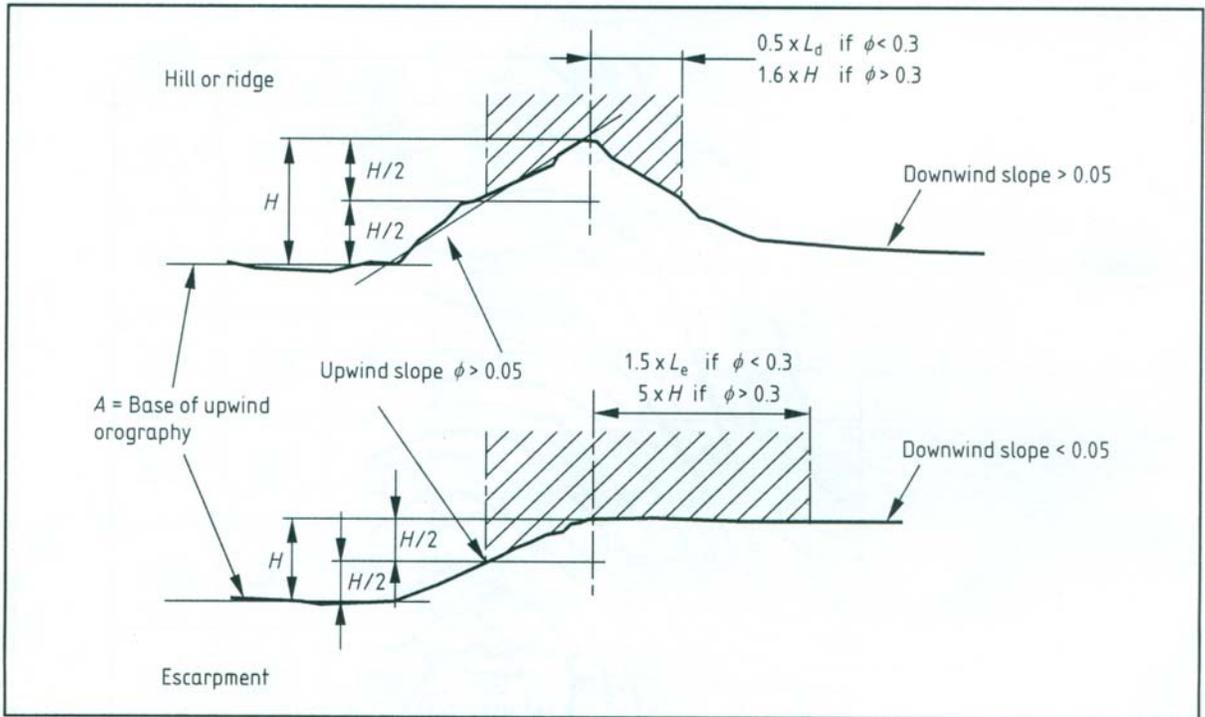
Figure 6: Definition of significant orography (Figure NA.2 of NA to BSEN 1991-1-4:2005)
