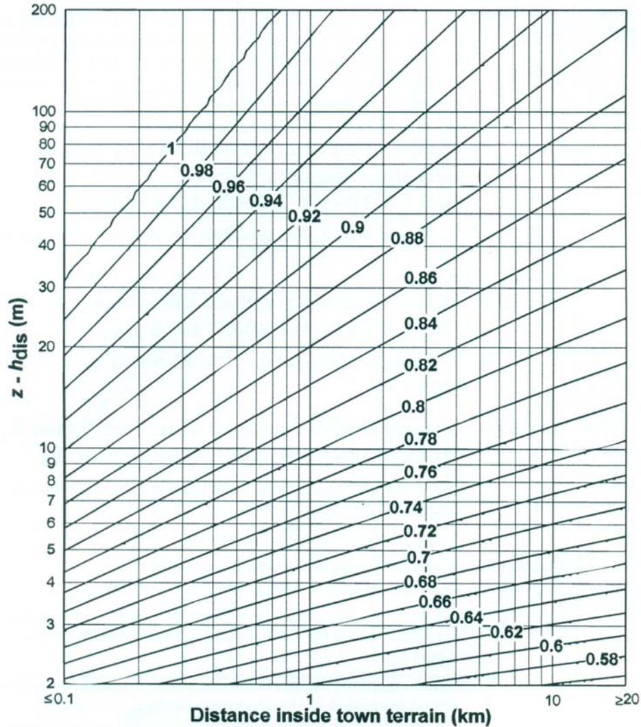
NOTE The height  $z$  is the height at which  $v_m$  is sought.
