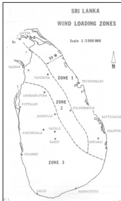
Figure 1: Wind zones map in Sri Lanka
