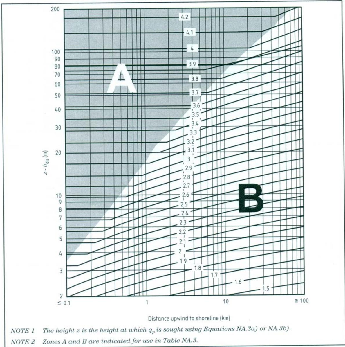
Figure 7: Values of exposure factor ( $c_e(z)$ ) (Figure NA.7 of NA to BSEN 1991-1-4:2005)
