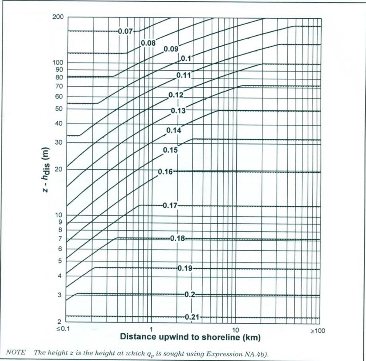
Figure 9: Values of turbulence factor related ( $I_v(z)_{flat}$ ) (Figure NA.5 of NA to BSEN 1991-1-4:2005)
