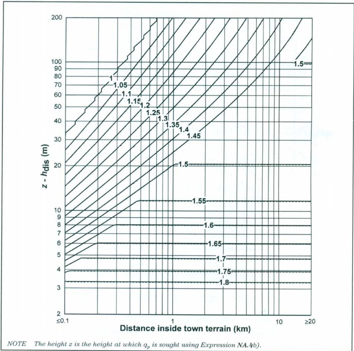
Figure 10: Values of turbulence correction factor  $k_{I,T}$  for town terrain (Figure NA.6 of NA to BSEN 1991-1-4:2005)
